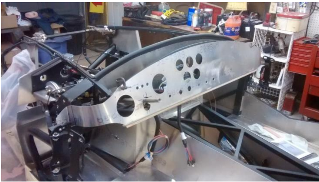
Installation of gauges into the dash
