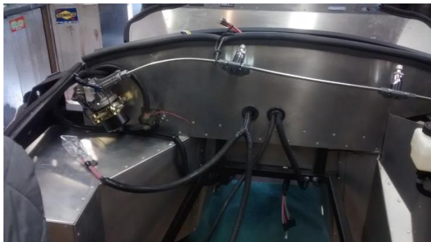
The back of the instrument panel and wiper motor installation.
